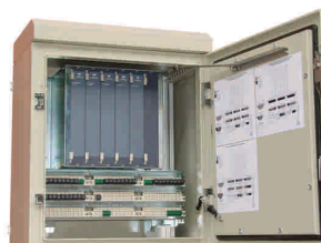
24/48 Port Remote† Description Model # 48 POTS/24 ADSL+POTS Cabinet 9501 in 24 ADSL+POTS mode: requires three 8 ADSL RT Card 9530 plus two 12 POTS RT Card 9562-L3 in 48 POTS mode: requires four 12 POTS RT Card 9562-L3 48 ADSL Cabinet 9501-L1 in 48 ADSL mode: requires six 8 ADSL RT Card 9530
